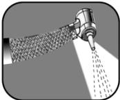
2) Turn on the turbine without using it for at least two minutes to drain the waterlines.
