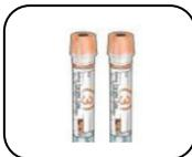
4) Close beaker on a plane surface. Take the Sample tube (NOT TO OPEN It) and firmly insert it in the opening with the cap to the bottom. The sample tube fills automatically. Bring out the sample tube as soon as it is filled. Reiterate the same operation with the second sample tube. Homogenize the contents of the sample tubes and preserve at room temperature until forwarding. After use, the cover in the lid of the beaker must be closed again using the round adhesive of safety.
