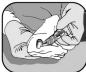
1) Perform water collection before or 2 days after the last treatment with antibacterial solution. Wash the outside of the turbine with antibacterial solution or with antibacterial wipe. Sterile gloves should be worn when collecting.
